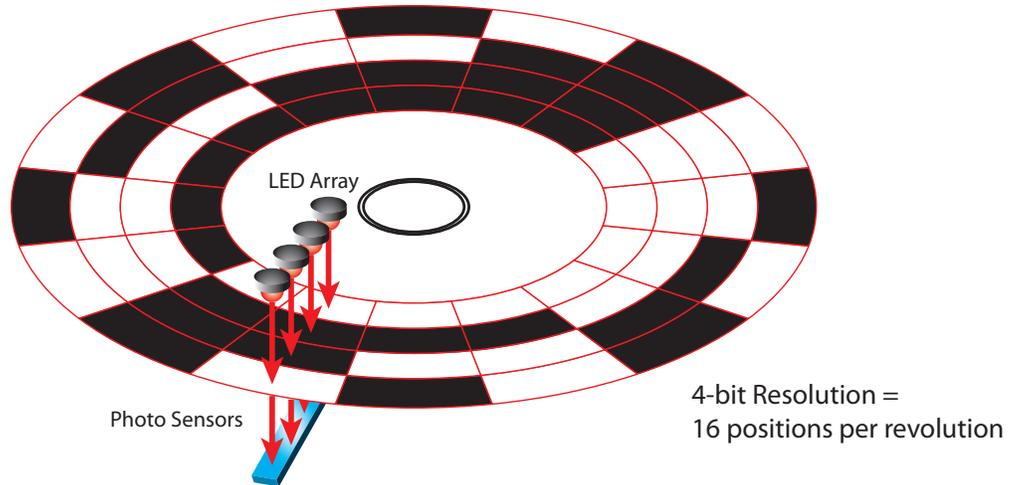
Resolution for absolute encoders is defined as the number of *positions per revolution* as the disk rotates through 360°. Sometimes the equivalent term *codes per revolution* is used.
