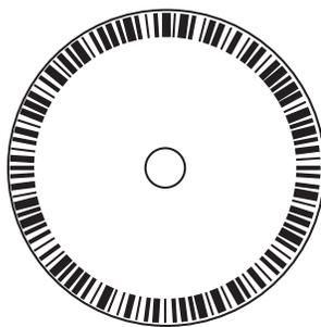
An absolute encoder with a bar code can offer programmable resolution: for example, a 12-bit encoder (4,096 positions per resolution) can be programmed to output from 2 to 4,096 codes per revolution.
