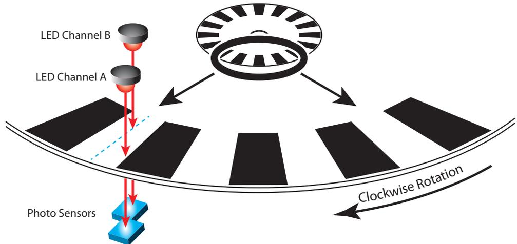
This yields a second output waveform, Channel B, shifted in phase from Channel A by 90 electrical degrees.
