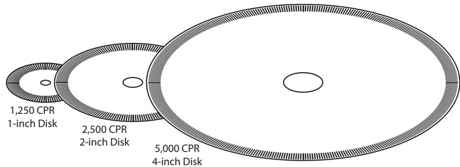
The drawing shows that, for traditional encoders, high resolution requires more lines on an encoder disk. If there's not enough space for the lines to fit, then the only solution is to make a bigger disk. To double the resolution, you have to double the disk's diameter.
