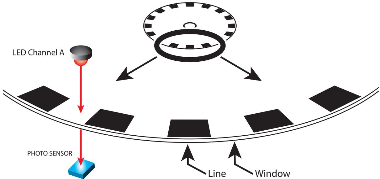
When an LED projects light at the disk, the light strikes either a window or a line. Windows allow light to pass through the disk to a photo sensor on the other side. Lines block the light. As the disk rotates, output from the encoder module—Channel A—is a series of high and low signals; their value depends on whether the photo sensor receives light (high) or not (low).
